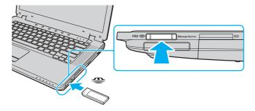
Be sure to hold the Memory Stick media with the arrow pointing in the correct direction as you insert it into the slot. To avoid damaging your computer or the Memory Stick media, do not force the Memory Stick media into the slot if you cannot insert it smoothly.
